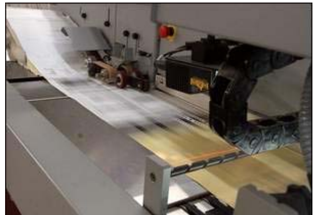
A machine at Databank scans paper records at a rate of 200 documents per minute and converts them into digital images.
